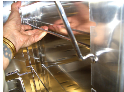
TILT THE RUNNER UP SLOWLY WHILE PULLING THE RUNNER OUTWARD AWAY FROM THE SIDE OF THE CABINET. DO NOT FORCE IT ASSURE BOTH SIDES ARE IN THE SAME POSITION AS YOU ARE LIFTING THE RUNNER
