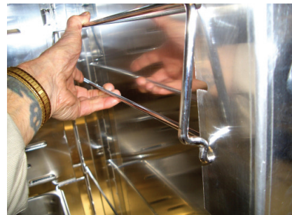
KEEP TILTING UNTIL THE RUNNER TOUCHES THE SLOTTED SIDE OF THE CABINET AND WITH BOTH ENDS OF THE RUNNER EQUAL DISTANT FROM THE CABINET SIDE THE RUNNER WILL SLIDE OUT EASILY. DO NOT FORCE IT
