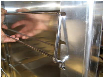
ROTATE THE RUNNER DOWN APPLYING A SLIGHT FORCE INWARD AGAINST THE RUNNER AND CABINET. DO NOT FORCE
